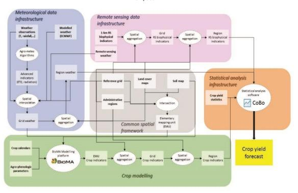
Figure 3 Data workflow among the M-CYFS system components to produce a final crop yield forecast Datasets are identified with boxes, whereas data processing is identified with ellipses
